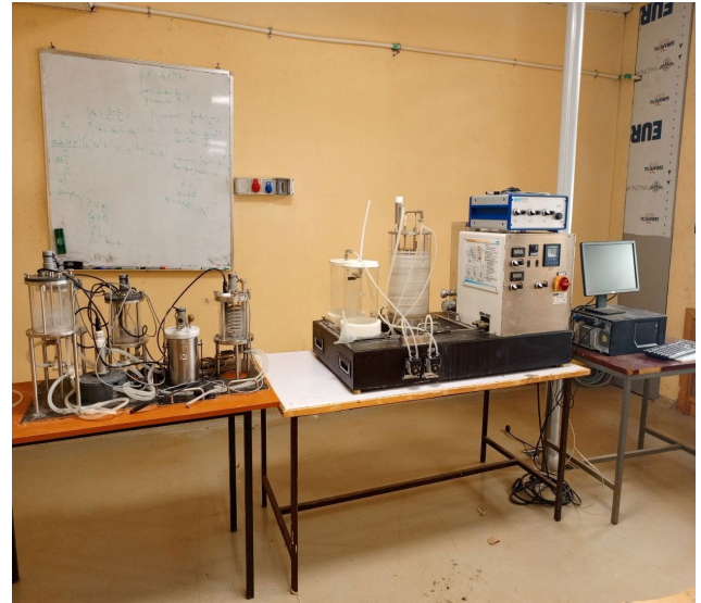
Gunt chemical reactor equipped with Tubular Reactor, stirred tank reactor, series and Batch Reactor
