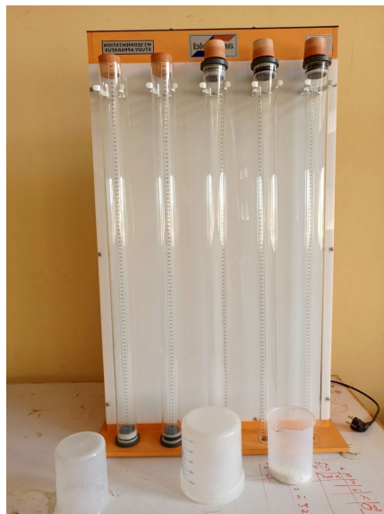
Batch sedimentation tank
