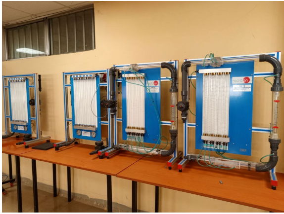
Flow meter demonstrator
