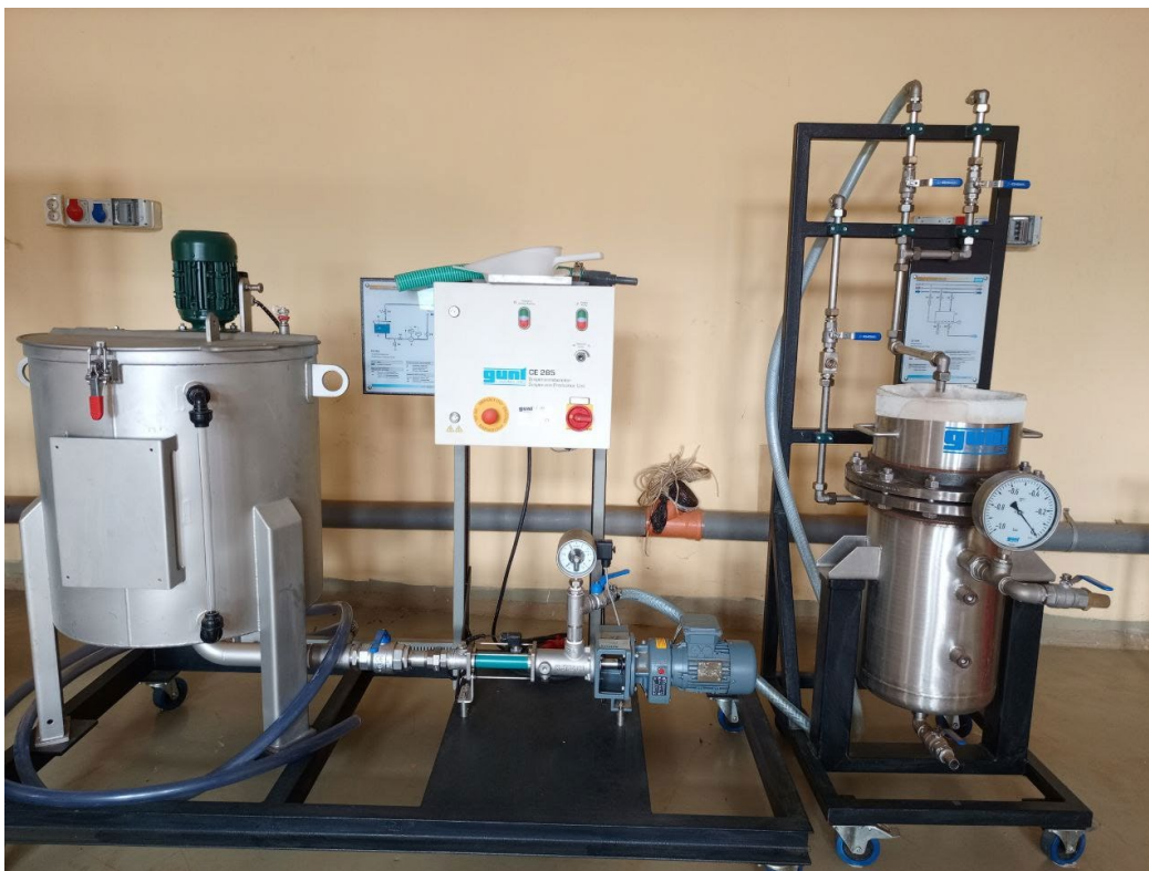
Suspension Production Unit equipped with Nutsch Vacuum Filter
