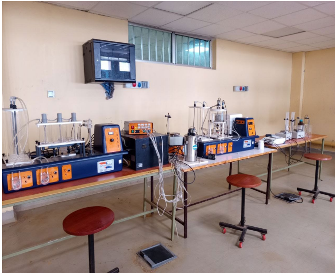
Armfilled chemical reactor equipped with Tubular Reactor, stirred tank reactor, series and Batch Reactor
