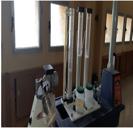
Fixed and Fluidized Bed Apparatus
