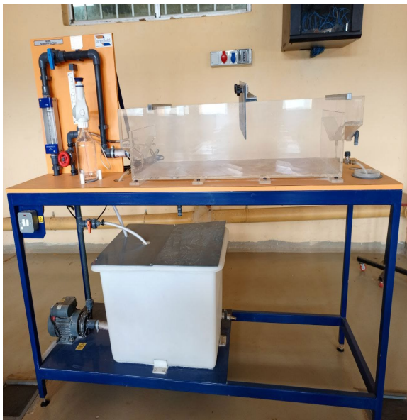
Continuous sedimentation tank
